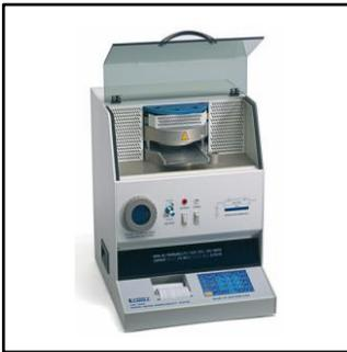
The 7000 water vapor analyzer range utilizes the sensitive and stable P2O5 sensor for absolute moisture measurement. These water vapor analyzers offer a wide measurement range of 0.002-1000 g/m<sup>2</sup>/day and precision temperature, humidity and flow control. Providing accurate and repeatable results for research and development testing of water transmission rate (WVTR) in both current and newly formulated packaging film materials and fast testing for Quality Control.
